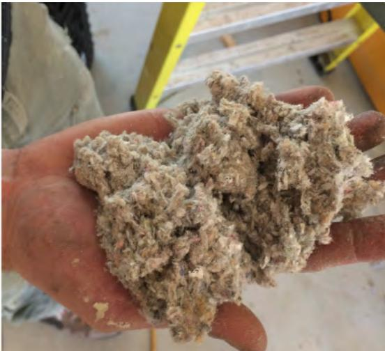
A wide variety of insulation materials are available, each of which has advantages for particular applications. When it comes to insulating walls and roofs—the primary components of the building enclosure—common options include cellulose, fiberglass, foam and mineral wool. Cellulose is Unity's go-to choice for these areas because of how it's made, how it's installed and how it performs.
