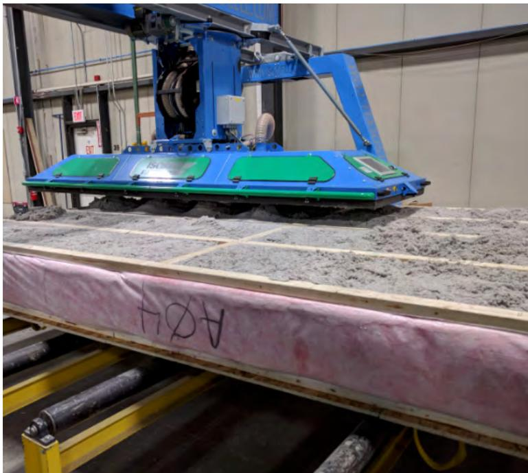
*Cellulose blown in through platen*
